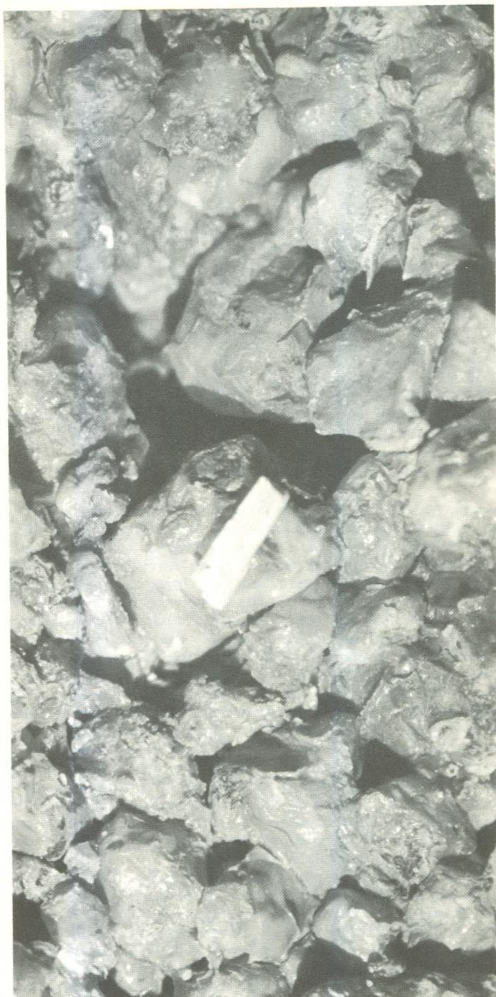
Figure 11.—Clay skins and bridges on sand. (Scale is 2 mm.)
