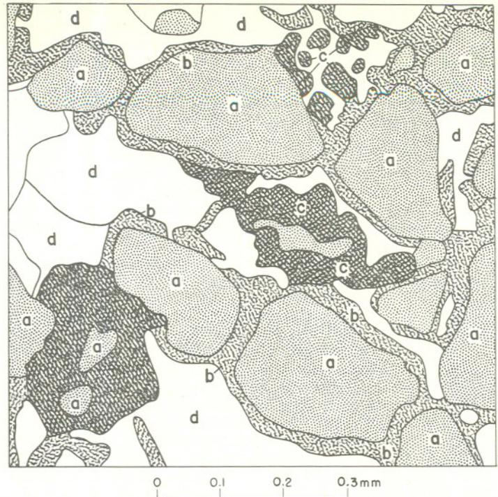
B, Diagram of thin section
