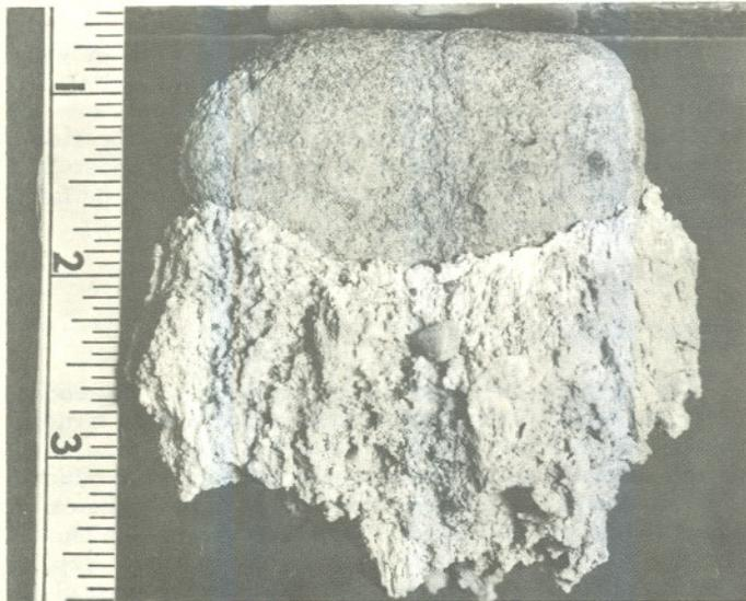
Figure 23.—Gypsum pendant formed below a small stone in a gypsic horizon.
