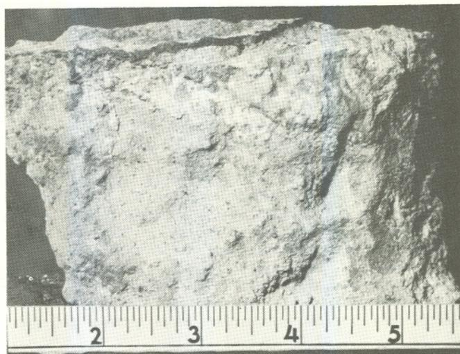
Figure 18.—Fragment of a duripan probably cemented with both lime and silica; thin, dark, extremely hard crust on upper surface is absent in some places. (Scale in inches.)
