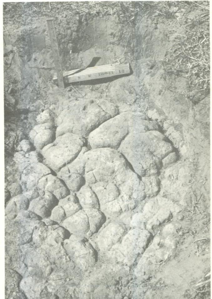
Figure 13.—Top, Natric horizon with columnar structure. Bottom, Bleached caps of columns.
