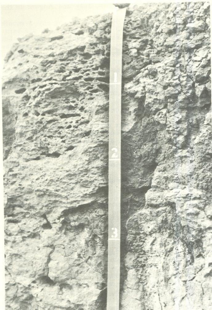
Figure 25.—Hardened, exposed plinthite. Large, rounded, tubular holes to left of scale presumably were at one time filled with clayey material that did not harden with rest of matrix. (Scale in feet.)
