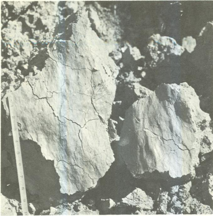
Figure 27.—Slickenslides from lower horizons of a Vertisol. (Scale in inches.)
