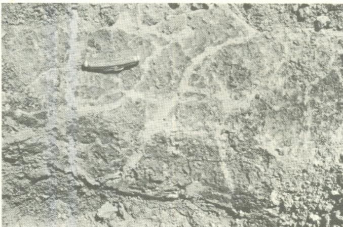
Figure 20.—Vertical and horizontal views of a fragipan: Top, Vertical view; ruler ticks are 6 inches (15 cm.) apart and upper boundary of fragipan is at 20 inches. Bottom, Horizontal view; knife is 3.5 inches (9 cm.) long.
