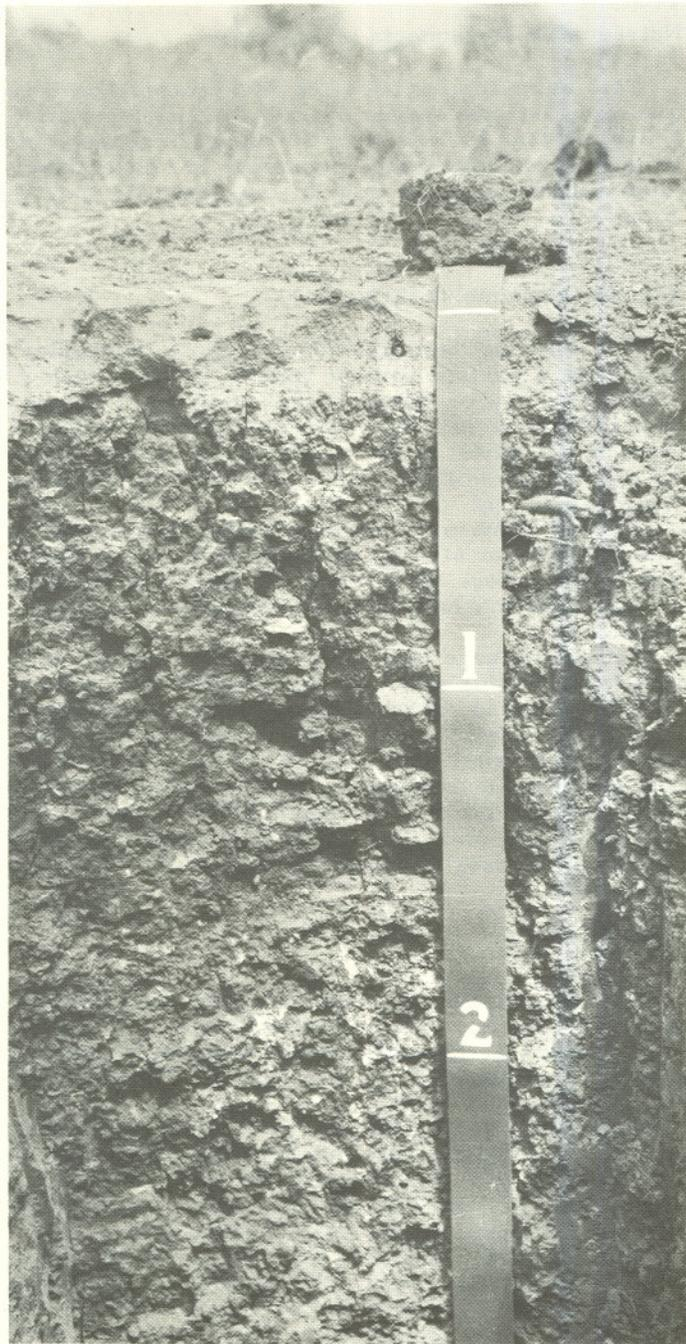
Figure 32.—Profile of a Mazaquert showing massive, light-colored crust at surface and, between 9 and 18 inches, wedges and parallelepipeds tilted from the horizontal.
