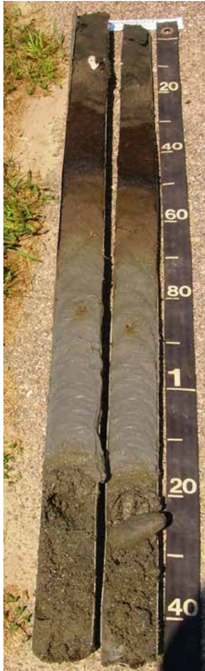
Profile of a Wassent exposed in a soil core from Rhode Island. Scale is in centimeters.
