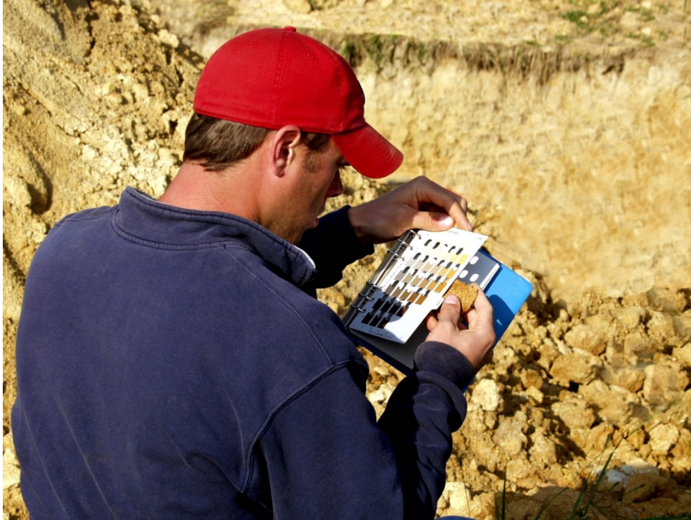
A soil scientist compares a hand sample from a horizon within a soil profile to a standard color chip in the Munsell Soil-Color Charts®. (Photo courtesy of John Kelley)
