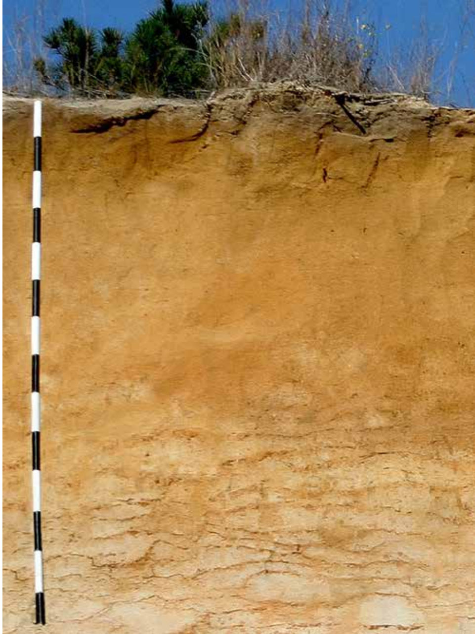
Profile of a Psamment (specifically a Quartzipsamment). This particular profile has lamellae (thin clay-enriched lateral bands) below a depth of about 90 cm. Scale is in 10-cm increments. (Photo courtesy of John Kelley)
