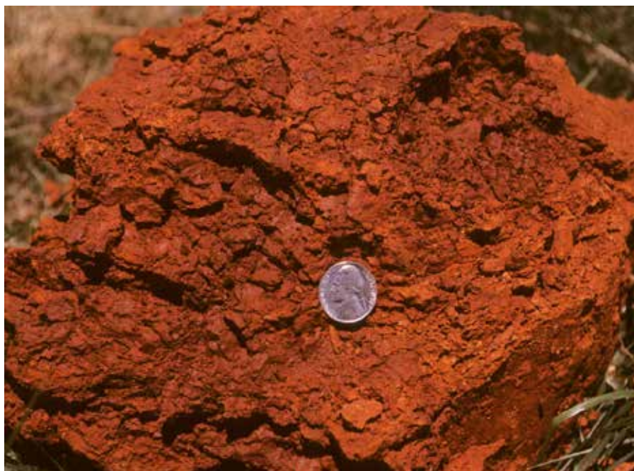
Clay films (slightly darker red) on surfaces of peds throughout an argillic horizon. (Photo courtesy of John Kelley)
