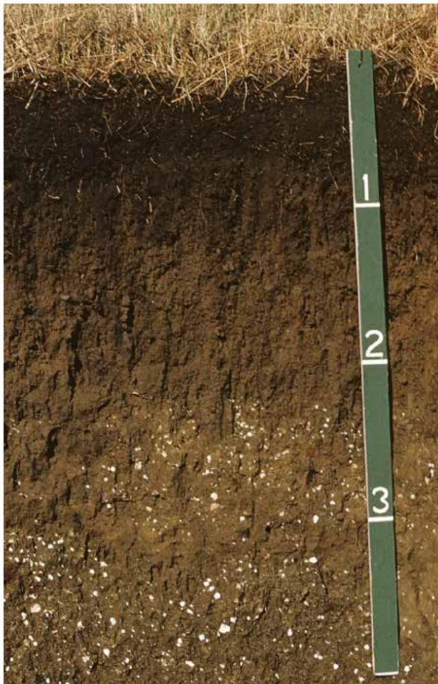
Profile of a Calciustoll with identifiable secondary carbonates (white bodies) below a depth of about 28 inches. Scale is in feet.
