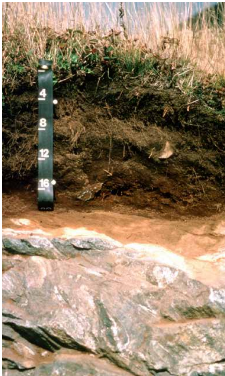
Profile of a Udept (specifically a Dystrudept) in North Carolina. Bedrock is below a depth of about 18 inches. Scale is in inches. (Photo courtesy of John Kelley)
