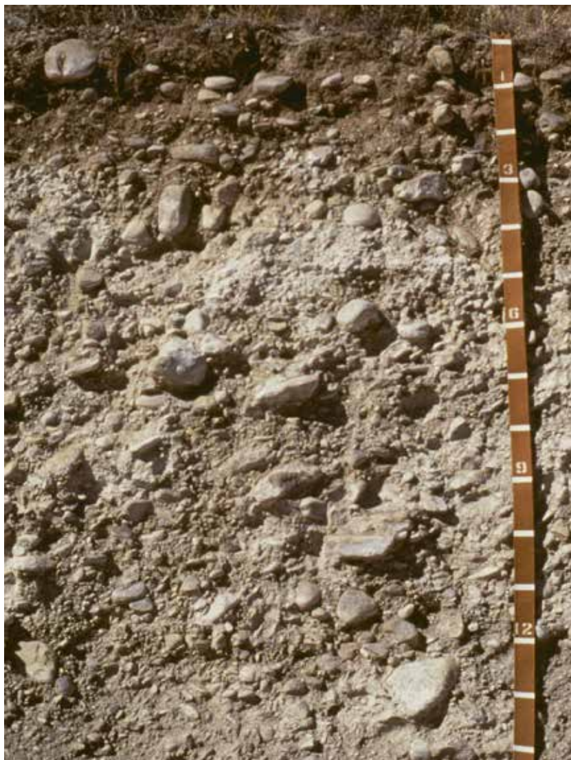
Profile of a Calcic (specifically a Haplocalcid). The white color below a depth of about 30 centimeters is due to accumulations of calcium carbonate. Scale is in decimeters.
