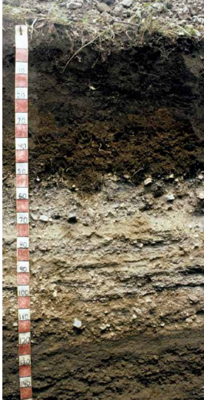
Profile of a well drained, gravelly Humustept in the Philippines. The soil formed in stratified layers of material, including volcanic ash. It has a dark, humus-rich umbric epipedon about 28 cm thick. Below this epipedon is a cambic horizon that extends to a depth of about 55 cm. Scale is in cm.
