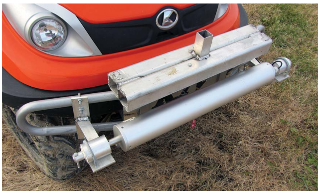
A vehicle-mounted passive gamma-ray sensor.
